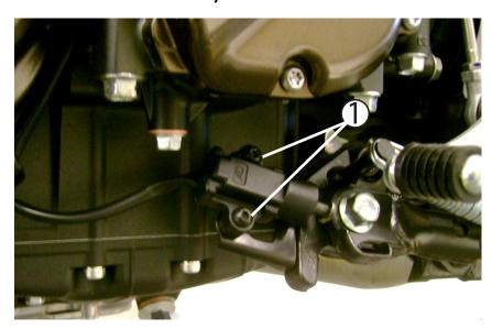
Using a 3mm allen tool and a 8mm wrench Remove the (2) OEM fasteners. You will reuse the (2) OEM nuts, so hang on to them.
