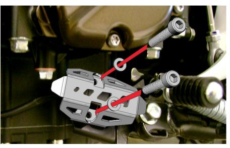
Now using a 8mm wrench and a 4mm allen tool, install the guard as shown using the OEM nuts and the 2 provided M5 x 25 socket head cap fastners.
